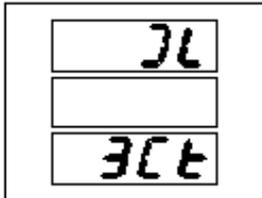
There are 2 options for the current wiring modes, i.e. “3C” referring to 3 CTs used for current wiring; “2C” referring to 2 CTs used for current wiring to calculate phase B current in three-phase balanced environment (some model numbers don’t support this option). The setting methods are as follows.
